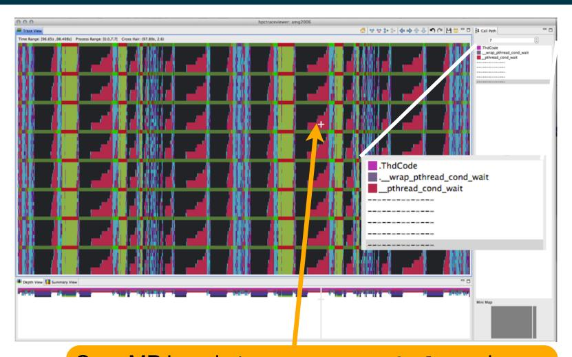
OpenMP loop in hypre\_BoomerAMGRelax using static scheduling has load imbalance; threads idle for a significant fraction of their time
