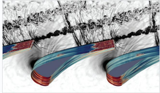
Flow in the transonic turbine inlet guide vane LS89 at  $Re=1.2$  million, computed using 4th-order-accurate DG. The acoustic waves and shock system are visualized via numerical Schlieren, whereas the instantaneous wall heat flux is shown on the suction side. Image: J. S. Cagnone, M. Rasquin, and K. Hillewaert, Cenaero.
