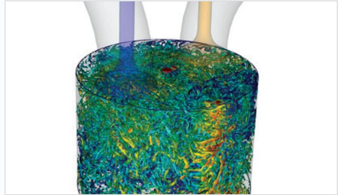
Snapshot of turbulent eddies in the compression stroke during the third engine cycle (1700.5 CAD). Eddies colored by velocity magnitude in the TCC-III internal combustion engine designed by GM. Image: Argonne National Laboratory
