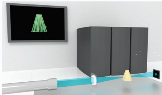
This illustration shows a coherent x-ray beam focused on a large-scale specimen while recording far-field diffraction patterns as the specimen is scanned and rotated. In the background is a computing system using automatic differentiation approaches to reconstruct a 3D image. Image: Ming Du, Argonne National Laboratory
