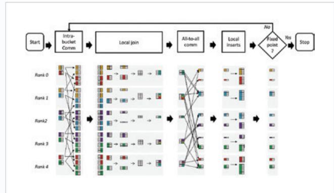
A diagram of the distributed hash-tree join algorithm highlighting the different stages and multiple levels of partitioning used to balance the workload. Image: Sidharth Kumar, University of Alabama at Birmingham
